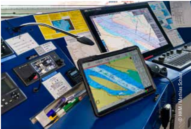
The Portable Pilot Unit (PPU) supports the pilots' work as an independent system.
