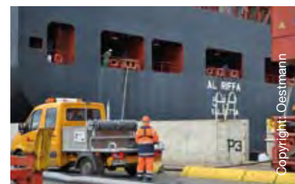
The linesmen's winches are mounted on a small truck
