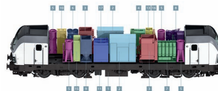
Engine room layout AC locomotive, high power
