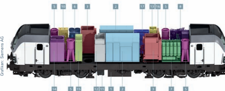
Engine room layout AC locomotive, high power
