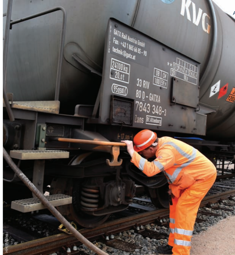
Railcar inspector Fred closely checks a tank wagon. He can see from the label that the car is carrying inflammable and environmentally dangerous goods.
