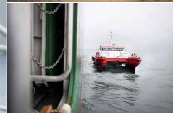
The pilots arrive in fast double-hulled boats bringing the portable pilot unit with them.
